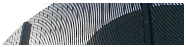
**Steelcraft 358** is a heavier-duty welded mesh for when security is paramount. The 4mm wires are set in a pattern considered both difficult to climb and to attack, with apertures too small for cutting tools, finger-holds or foot-holds.
